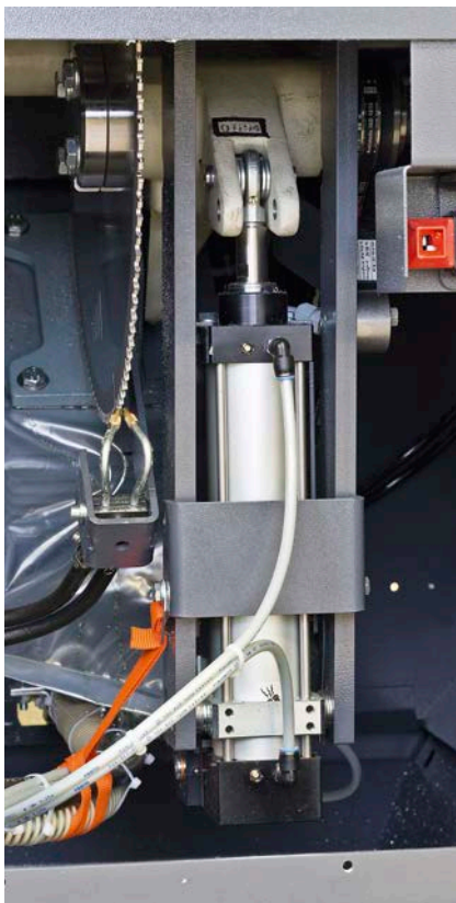
Hydro-pneumatic blade feed.
