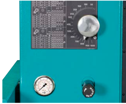
Clamping pressure reduction for thin-wall materials.
