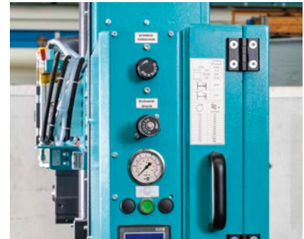
Infinitely variable hydraulic sawband feed.
