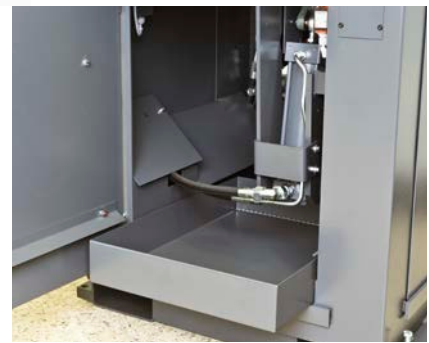
Large front door affords easy access for blade changes and chip tray removal.
