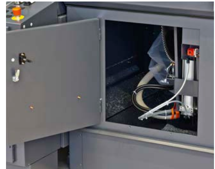
Large door provides easy access for blade changing and maintenance.
