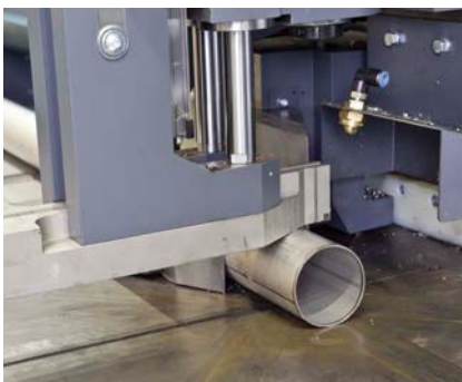
Programmable automatic pressure reduction via proportional valve to process thin-wall tubes and special profiles (only on KKS 463 NA).
