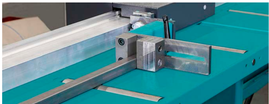
L 42 P 'pusher' length measuring system, which can also operate as a traditional back stop.
