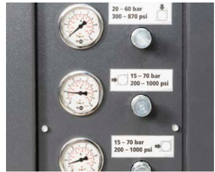
Adjustable clamping pressure for cutting thin-wall tubes and profiles.
