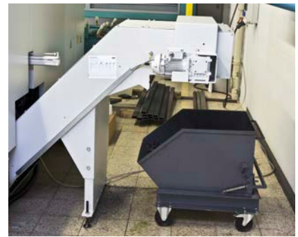
Hinged belt chip conveyor to remove chips, trims, slugs and remnants (only on KKS 463 NA).
