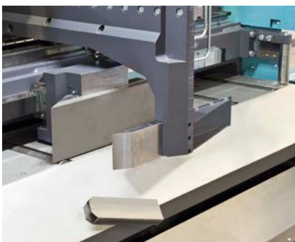
Outfeed sorting gripper holds material during the cut and sorts trims, remnants and good parts to pre-programmed positions.
