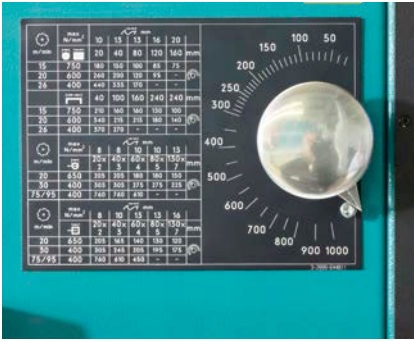
Infinitely adjustable feed rate to a chart.
