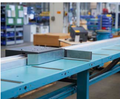
L 42 P 'pusher' length measuring system, which can also operate as a traditional back stop.
