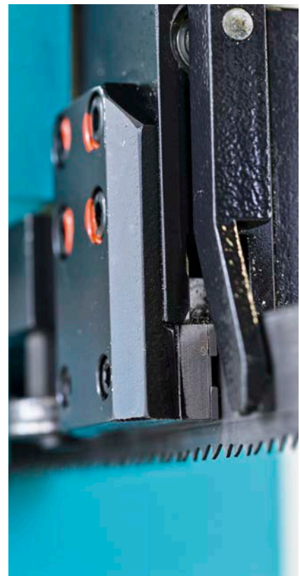
Carbide band guides for precise cuts.
