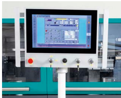
Pendulum-mounted touchscreen control panel.
