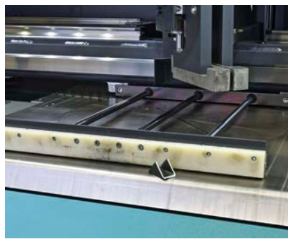
Integrated brush-off system to remove trims and remnants, slugs and chips from the table.
