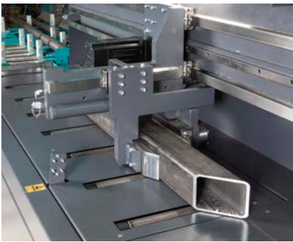
Precision positioning of material via shuttle feed gripper running in dual linear guides.
