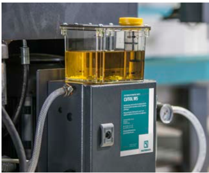
Atomiser lubrication for virtually dry parts.
