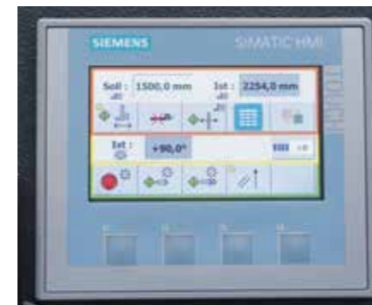
L 42 NC length measurement device Easy operation and programming on the sawing machine.
