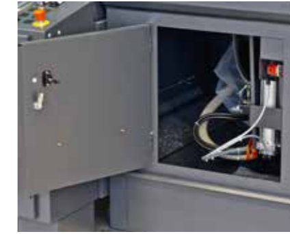
Large front door for rapid saw blade change and easy maintenance.
