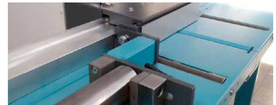
L 42 P automatic material feed and length stop Can be used as length stop or pusher plate.
