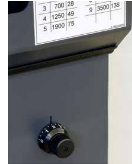
Feed regulator for universal, infinitely variable adjustment even during the sawing process.
