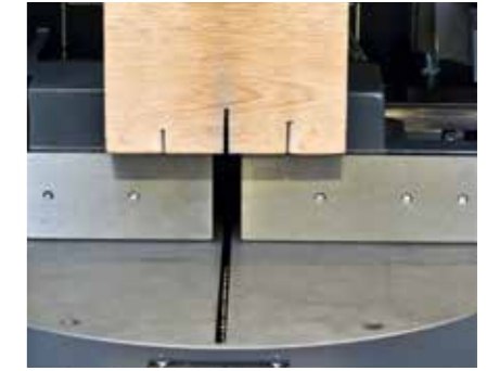
Vertical hardwood clamping block to protect material surface.
