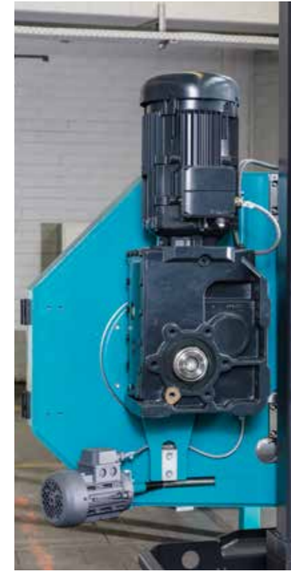
Heavy duty frequency-controlled geared motor.
